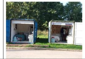
Purchase and fit out of 2 identical containers to demonstrate the benefit of fitting domestic or commercial sprinklers. The containers needed to be boarded out, and then cleared and reboarded by external builders after 3 separate burns.
